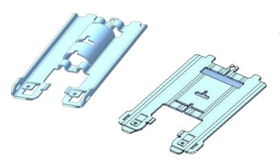
KOMPAS-3D rich collection of sheet metal modeling functions include bends, holes, louvers, fillets, punching (stamping), cuts, and cap closing of sheet metal bodies.
