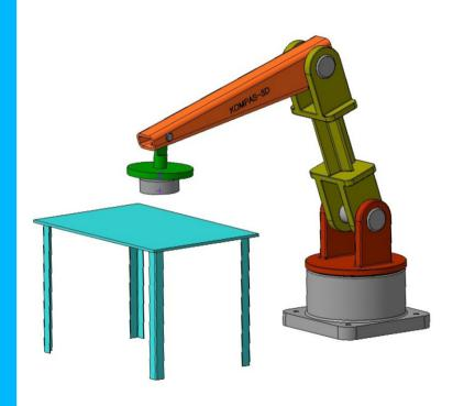
The Animation add-in performs motion simulation of 3D products developed with KOMPAS-3D. The types and parameters of part motions include velocity, rotation frequency, and duration.
